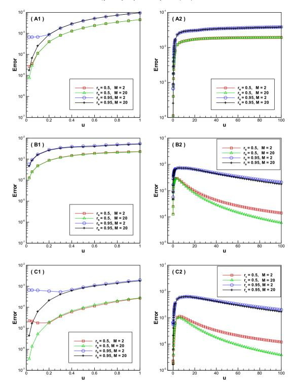
**Fig. 2.** Accuracy comparison for the methods vs.  $u = \lambda a$  where *a* is fixed to be 1. A, B and C, respectively, represent the original method, the new method without correction term and the new method with one constant correction term. Left:  $u \in [0, 1]$ ; right:  $u \in [0, 100]$ .
