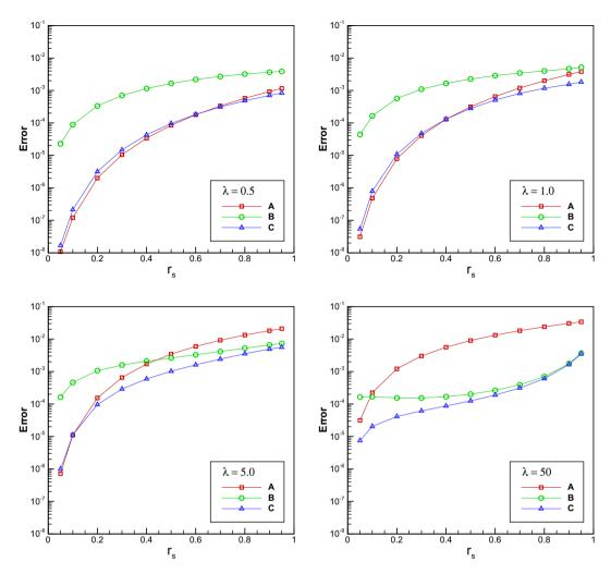
**Fig. 1.** Accuracy comparison for the methods vs. the source location *r*<sub>s</sub>. A, B and C, respectively, represent the original method, the new method without correction term and the new method with one constant correction term.
